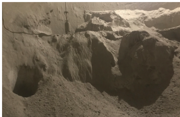
Clogging would quickly build up to a spilling point, so workers need to enter the vessel to clear it.
