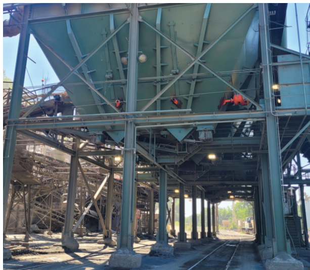
Tilcon's air cannons are strategically placed for optimum effect when fired in a sequence.
