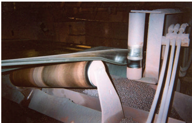
Figure 6 - Brute force tracking devices treat the symptoms rather than the root causes of mistracking, often result in belt edge damage.
