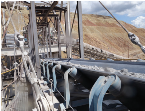
Conveyors are getting longer and meaning more exposure to vibration and wind.
