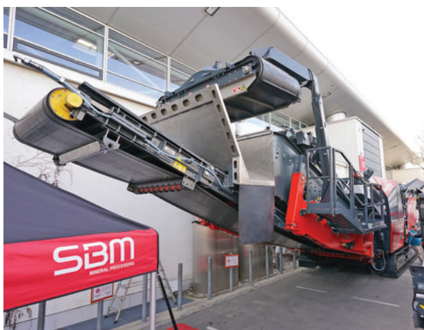
With double magnets and a 6 m wide secondary screen, the REMAX 600 large impact crusher's maximum capacity of 600 t/h can be fully utilised for the production of defined fines.
