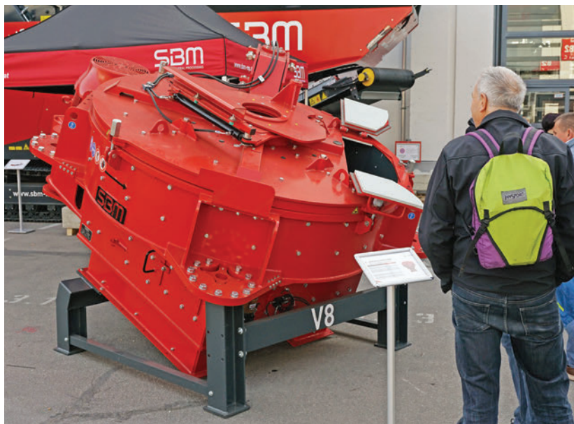
SBM presented the V8 vertical shaft impact crusher (VSI) as an economical solution for the production of high-quality sands.
