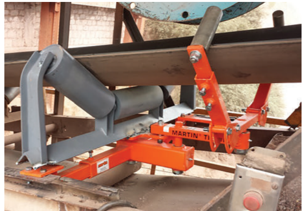
Figure 8 - Multi-pivot belt trainers use a torque-multiplying system to improve belt path correction. Copyright © Martin Engineering 2025
