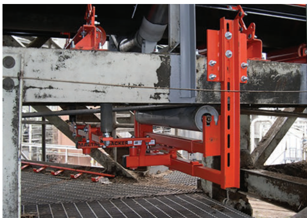
Figure 7 - The in-line sensing roll trainer has a carrying roll on a central pivot bearing with vertical guide rolls mounted on both sides. Copyright © Martin Engineering 2025
