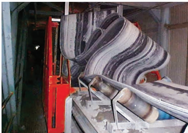
Figure 3 – Contact with the structure can break mechanical splices with expensive consequences. Copyright © Martin Engineering 2025
