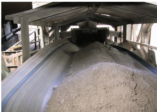
Figure 1 – Contact with the support structure can cause serious belt damage. Copyright © Martin Engineering 2025
