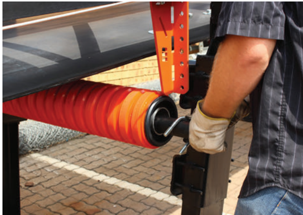
Figure 6 - This roller tracker uses a unique ribbed lagging made of durable polyurethane to increase performance. Copyright © Martin Engineering 2025
