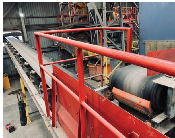
The Pit Viper cleaning blade can be replaced without any tools by removing and reinserting a single retaining pin (shown bottom right of picture).
