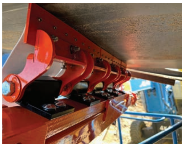
Cartridges with individual tensioning improves cleaning efficiency and effectiveness.
