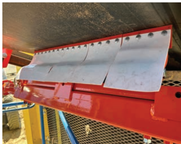
Slick heavy duty deflector shields improve performance from wet applications that experience buildup.
