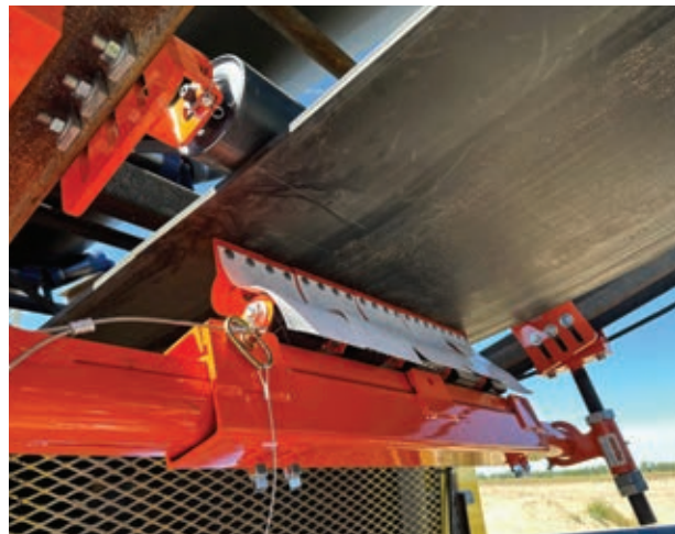
The mounting assembly firmly secures the secondary cleaner to the stringer.
