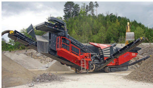
With 600 tph and up to five end products, the SBM REMAX 600 redefines mobile crushing in the 80-tonne class.
