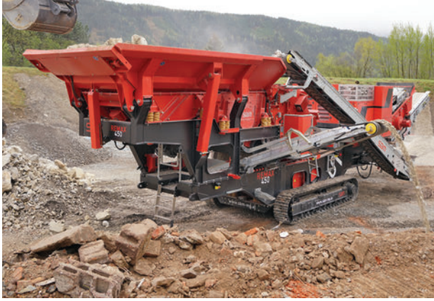
With pre-screening and an optional 2-deck production screen, the SBM REMAX 450 impact crusher delivers high quality end products directly on the construction site.
