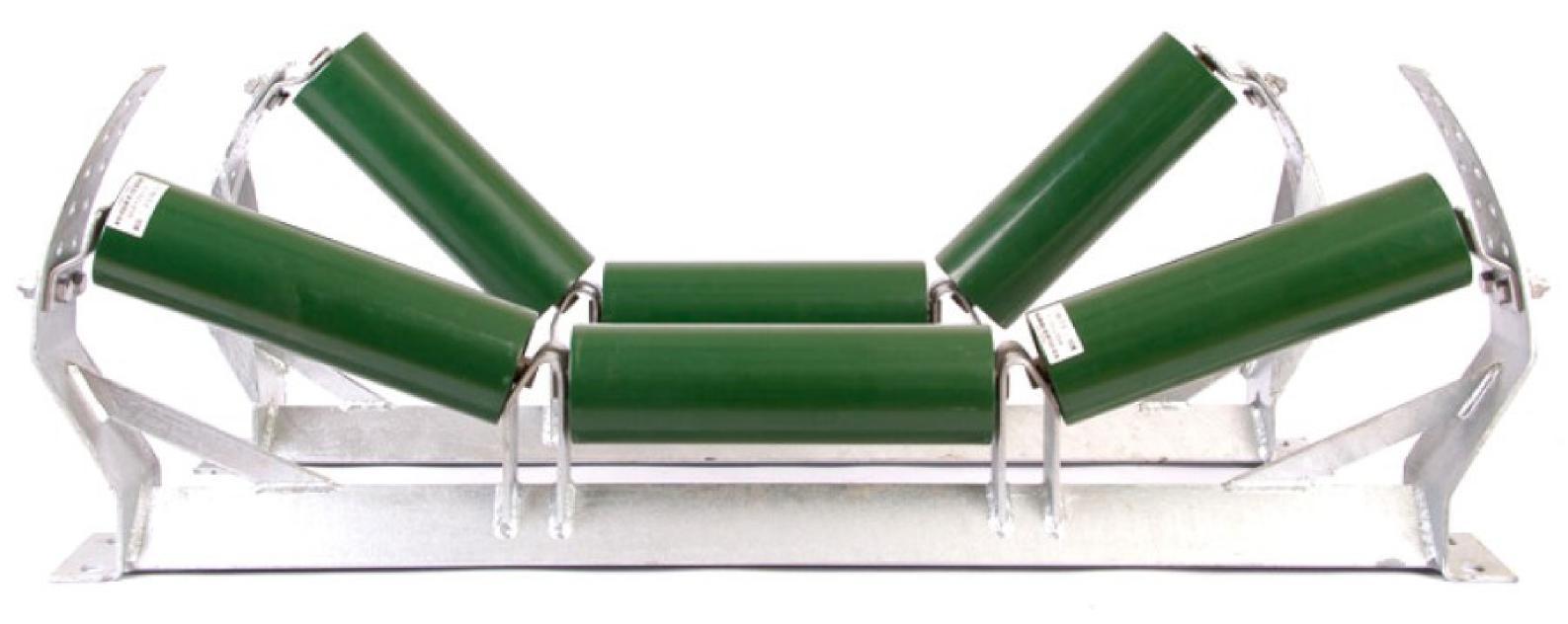
Transition frames are galvanised to 140 microns and are adjustable from 20 to 45 degrees in 5-degree increments.
