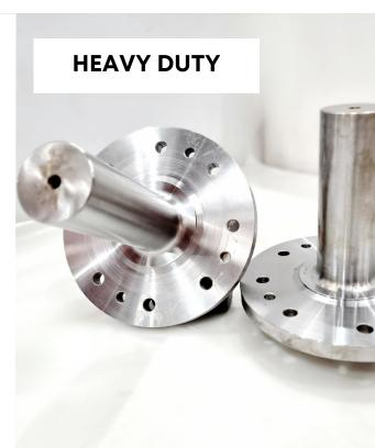
Drums and shafts are available in standard and heavy-duty, the standard range of drums comprise of diameters from 200-400mm with heavy duty comprising of 324-500mm, standard shafts from 30-70mm diameter and heavy-duty from 60-100mm diameter, all drums are manufactured complete with heavy-duty through tubes for the shaft location thus creating a "through shaft".
