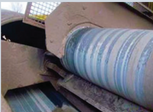
The existing metal blade delivered poor cleaning performance, while damaging the belt and splice. Copyright © 2023 Martin Engineering
