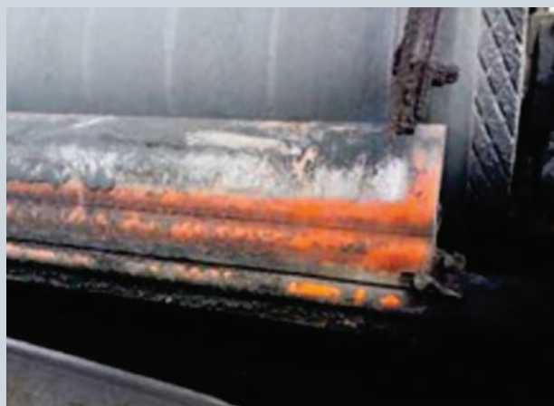
Martin blades' patented design creates a tight seal, flows easily over splices and maintains cleaning performance through all stages of blade life. Copyright © 2023 Martin Engineering
