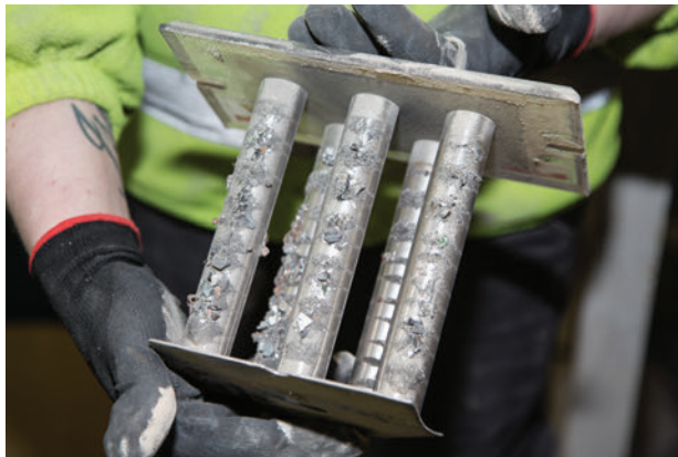
Figure 1 - Ferrous metal in recycled plastic captured on Tube Magnets
