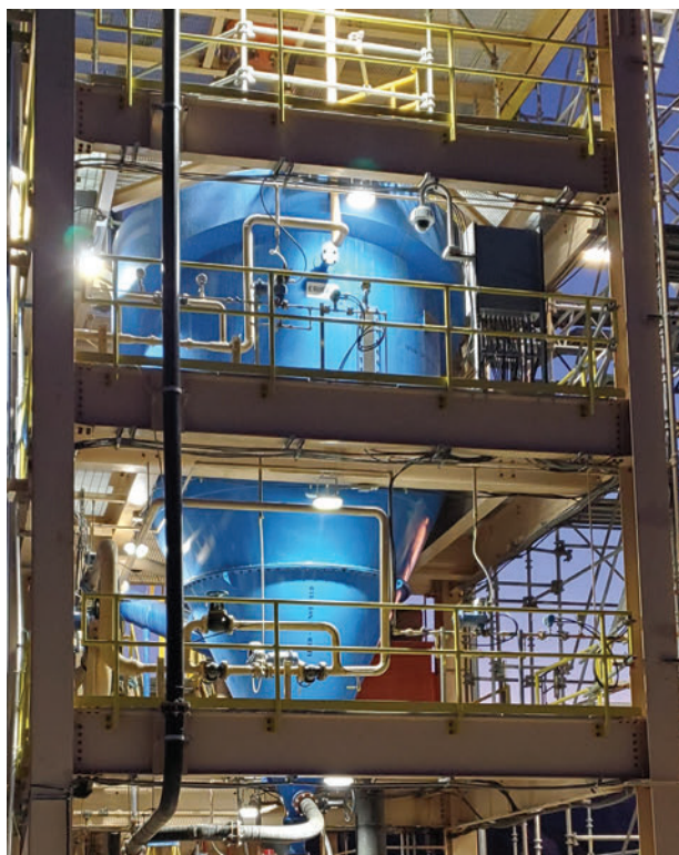
Using a novel aeration system to disperse fine bubbles into a fluidized-bed environment, the HydroFloat® Separator significantly increases the selective recovery of coarse particles by applying flotation fundamentals to gravity separation.
