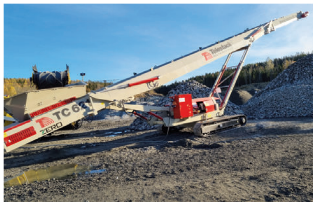
The TC621 tracked conveyor from the Telestack Zero range! Available in a range of power options, (diesel hydraulic, hybrid, dual power, electric-driven or battery operated), the Telestack offering enables companies who see the value in moving towards a more sustainable energy source. The benefits are many including the reduction in fuel consumption ensuring better operational efficiency, the reduced environmental impact and a much safer site with reduced vehicle movement.
