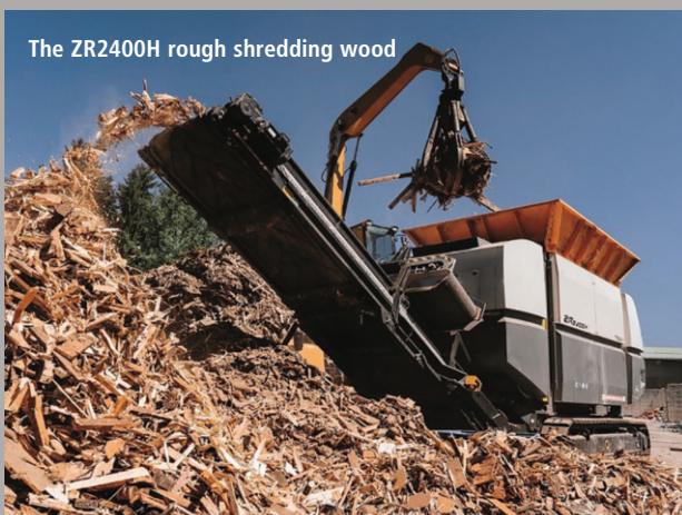
The machine’s low speed, high torque drive means it can process severe duty applications with ease
