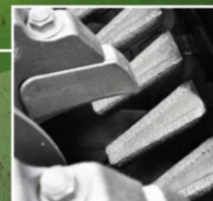
COUNTER KNIVES ENSURE LONGER AND TROUBLE-FREE SHREDDING.
