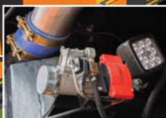
CLEANFIX SYSTEMS AUTOMATIC CLEANING OF THE HYDRAULIC OIL AND ENGINE COOLING.
