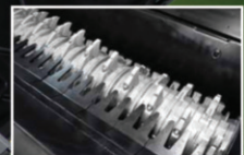
SINGLE SHAFT WITH MAX. 27 RPM.
