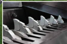
STANDARD SHAFT WITH CHANGEABLE CUTTERS FOR EASE OF MAINTENANCE.
