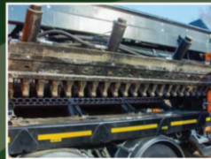
SHREDDING CHAMBER EASILY ACCESSIBLE FOR CLEANING OR CHANGING COUNTER KNIVES.
