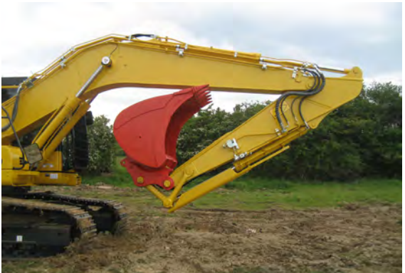
fig 1.4 Miller Scoop Bucket and Miller Coupler in transit mode
