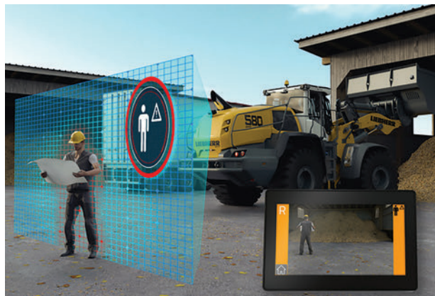
The Liebherr brake assistant automatically decelerates the wheel loader the moment the active personnel detection identifies a source of danger in the rear area.
