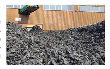
The main raw materials in a tyre are rubber, steel and textile fibres, which can be recycled for either the material or the energy it contains. Rubber and steel are both recoverable and can be used in various ways - steel is removed from the tyre until there is only rubber left and Turmec specialises in recycling solutions that shred the remaining material of tyres of up to a diameter of 3 m, down to a particle size ranging from 80 to 150 mm.
