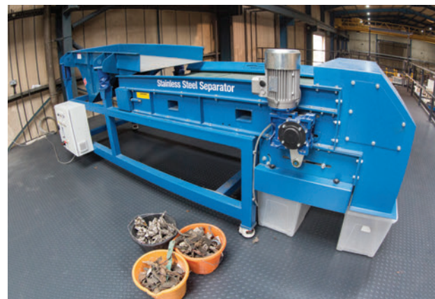
Figure 2 - An installed SSSC Magnetic Separator
