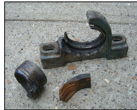
Example of Bearing Failure
