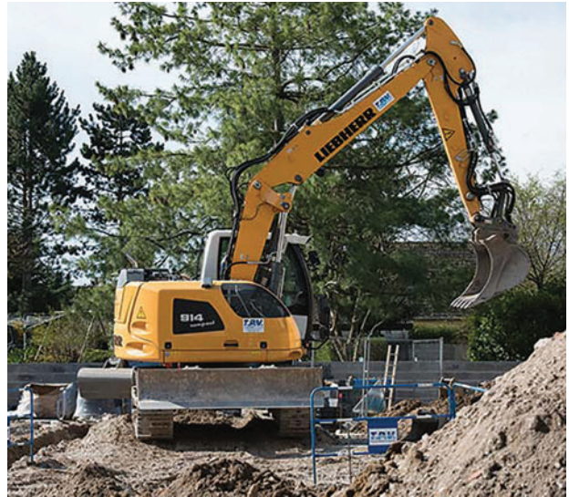
The Liebherr R 914 Compact crawler excavator with an operating weight of approx. 14 tonnes has a Stage IV / Tier 4f engine delivering 90 kW / 122 HP.
