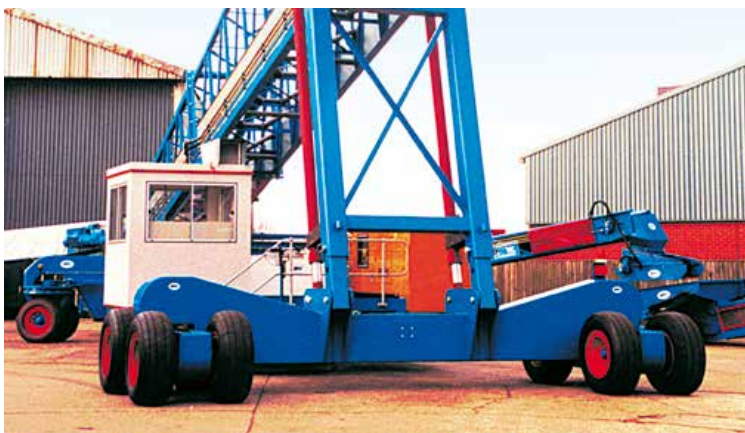
Forward axle beam with telescopic boom supports
