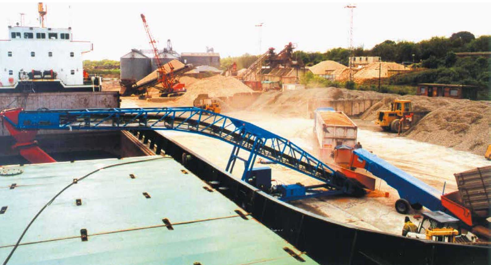
Feeder Conveyors discharge to the Shiploader
