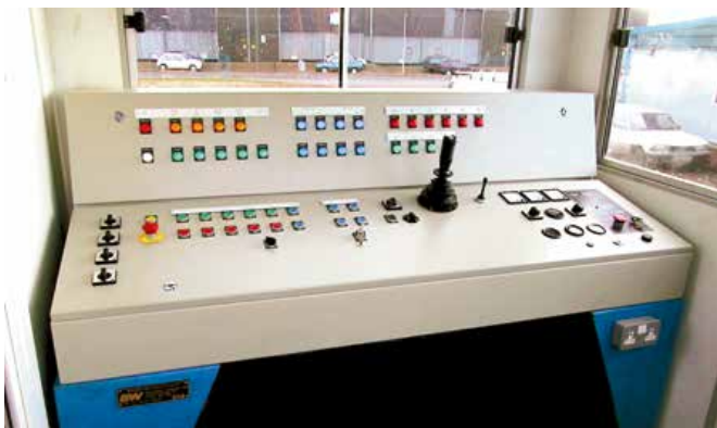
Full operator's control desk with joy-stick steering system
