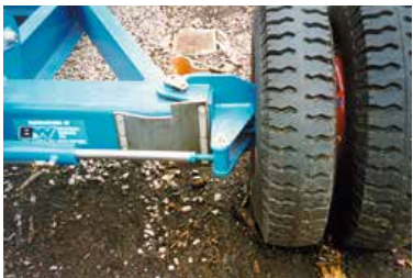
Tail end castor-wheel mounts with parallel push travel
