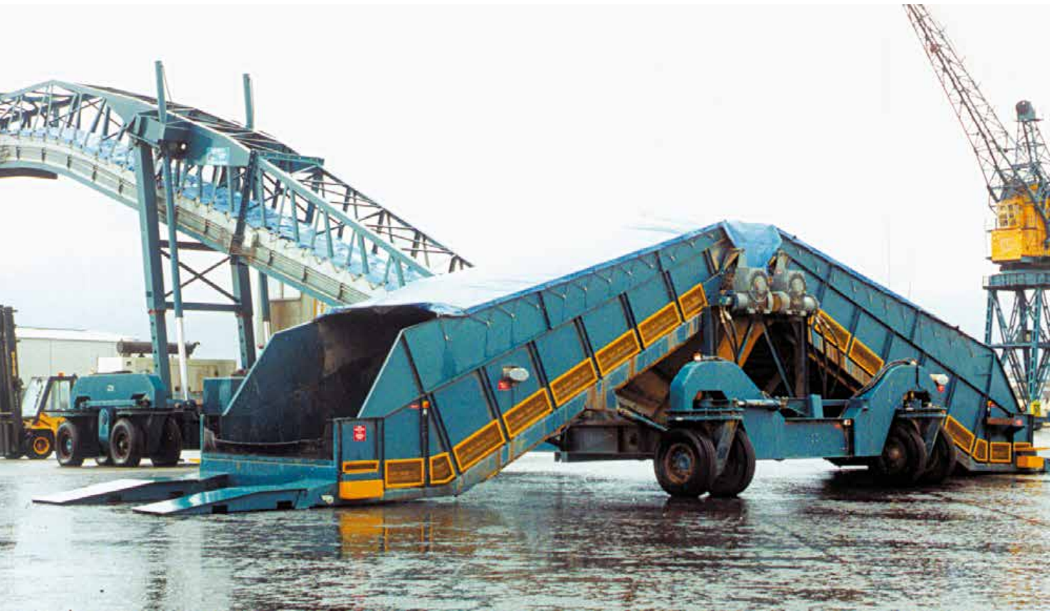
Twin Samson® Material Feeders with flexible enclosures
