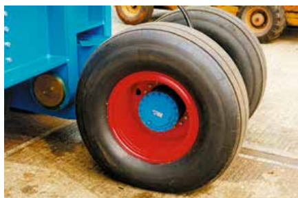
Integral hydraulic hub motor
