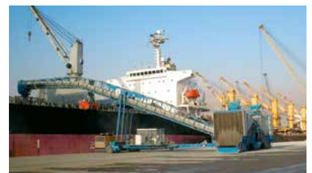
Shiploader with Twin Samson® loading Panamax vessel
