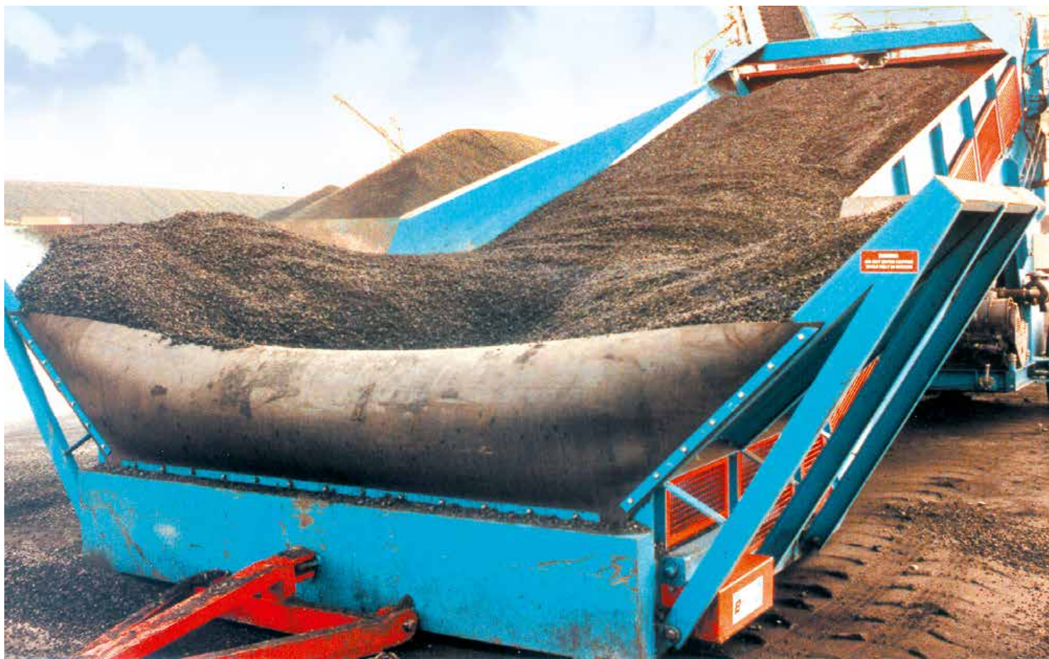
Stormmajor® receives coal from loading shovel for stockpiling and barge loading
