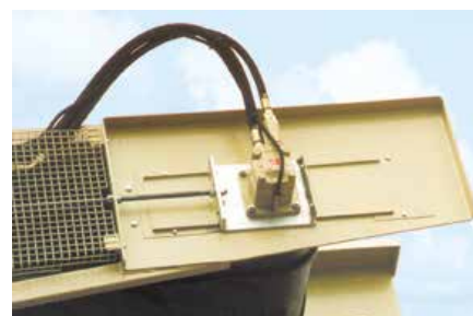
Drive to the head of the outloading boom conveyor with integral Danfoss type
