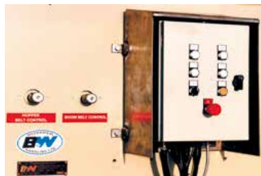
External control panel for diesel motor drive showing local engine key switch starting control without full instrumentation
