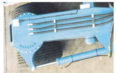
Hydraulic Actuator Steering System with slewing ring mounting for the twin wheel units.
