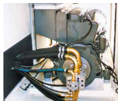
Diesel motor drive with triple section hydraulic pump system fitted to the side of the main chassis within a sound attenuated enclosure
