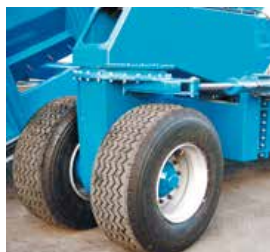
Twin Axle Steering Bogie with potentiometer alignment system to achieve Ackerman steering without a mechanical linkage.
