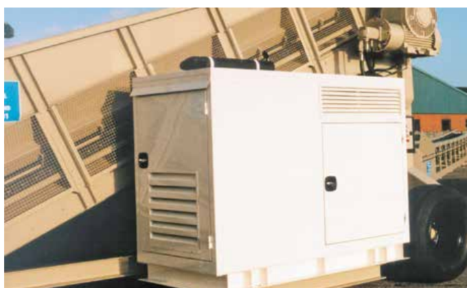
Diesel motor drive with triple section hydraulic pump system fitted to the side of the main chassis within a sound attenuated enclosure
