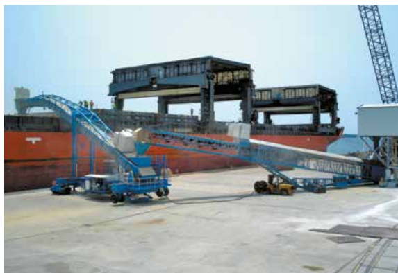
Shiploader – Conveyor Feed
