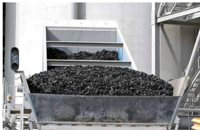
The Samson® Material Feeder supplied with a screw mounted across the discharge to meter the tyre chips to a vertical bucket elevator discharging to a high level bunker
