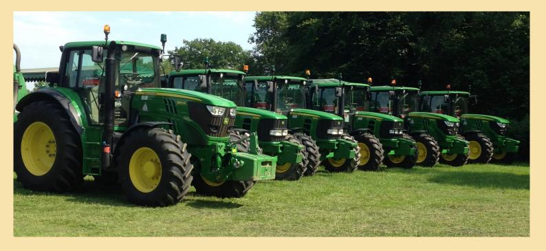
**John Deere 6105M**— 105hp— 4 cylinder turbo engine—420/85R38 rear & 380/85R24 front wheel equipment—16/16 power quad plus
