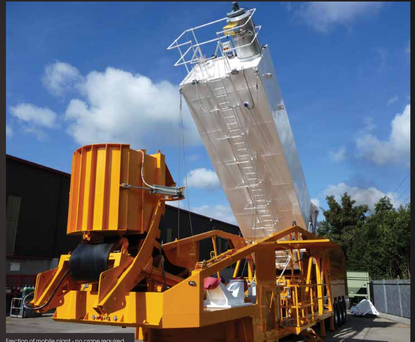
Erection of mobile plant - no crane required
