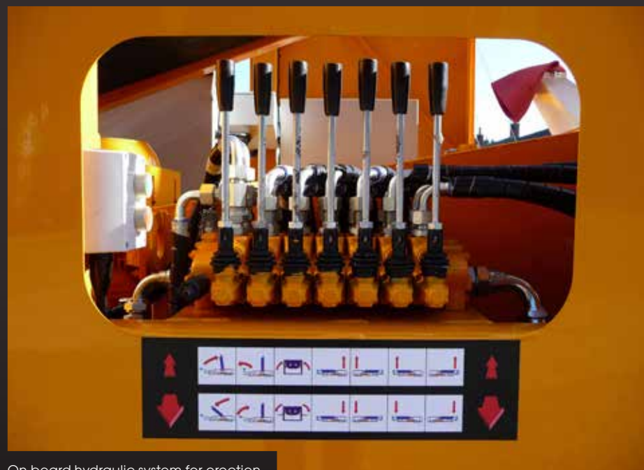
On board hydraulic system for erection
