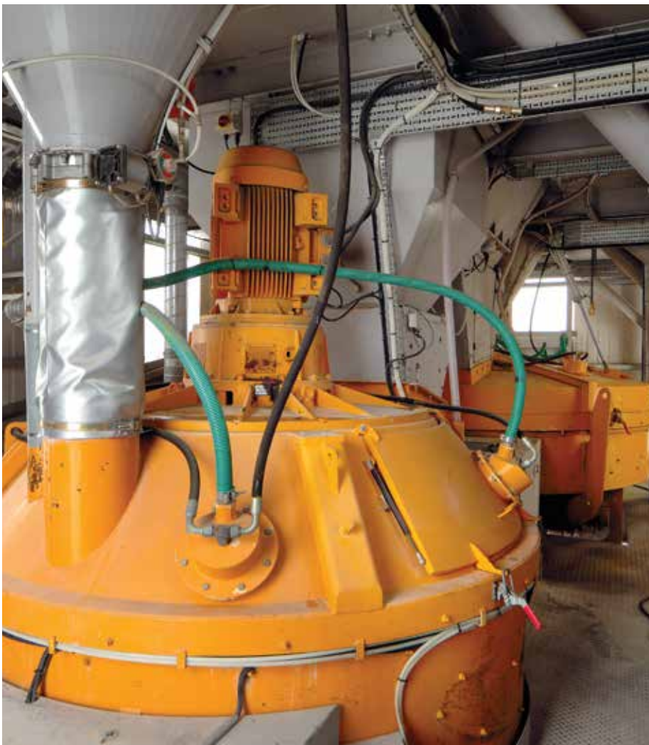
Single star mixing action. RP375 to RP750
