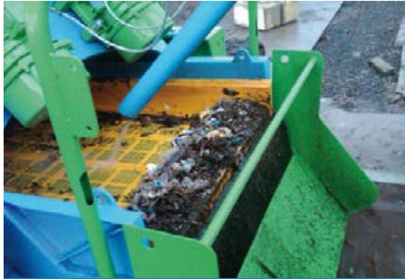
“ This unit integrates several processing phases including attrition, trash removal, dewatering and sizing of the clean recycled aggregate. ”
