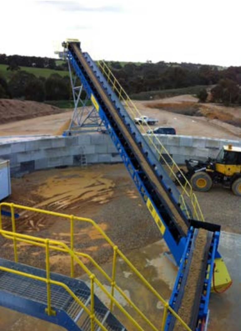
Both the dewatered silica sand and concrete sands are subsequently stockpiled using 26m radial conveyors which ensure a stockpile capacity of 5000 tons.
