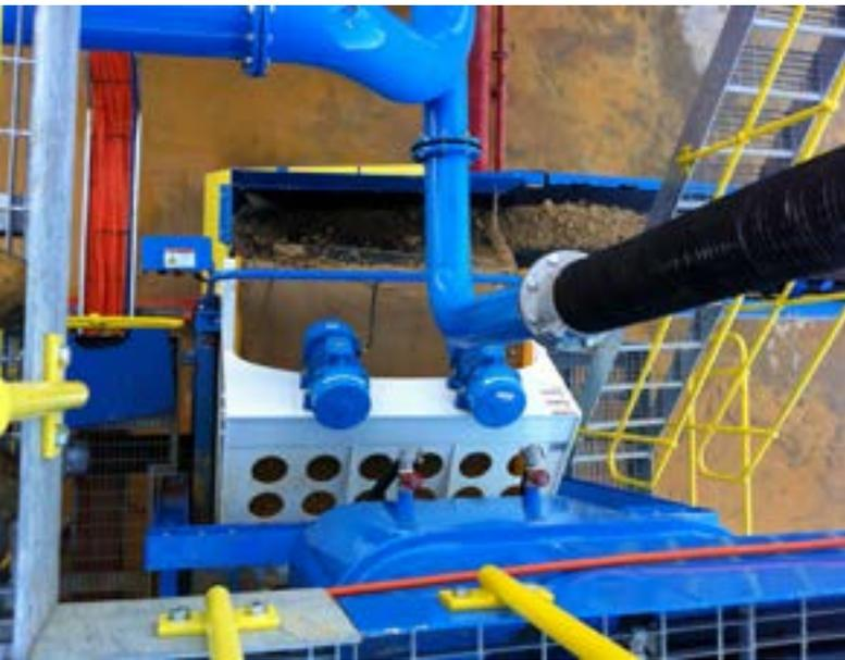
The underflow from the cyclone is delivered to the EvoWash dewatering screen before being transferred to the attrition cells.
