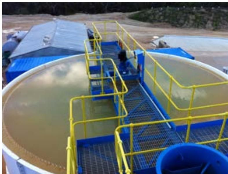
Waste water from the plant is processed by the AquaCycle thickener which recovers 90% of the water for re-circulation around the washing plant.
