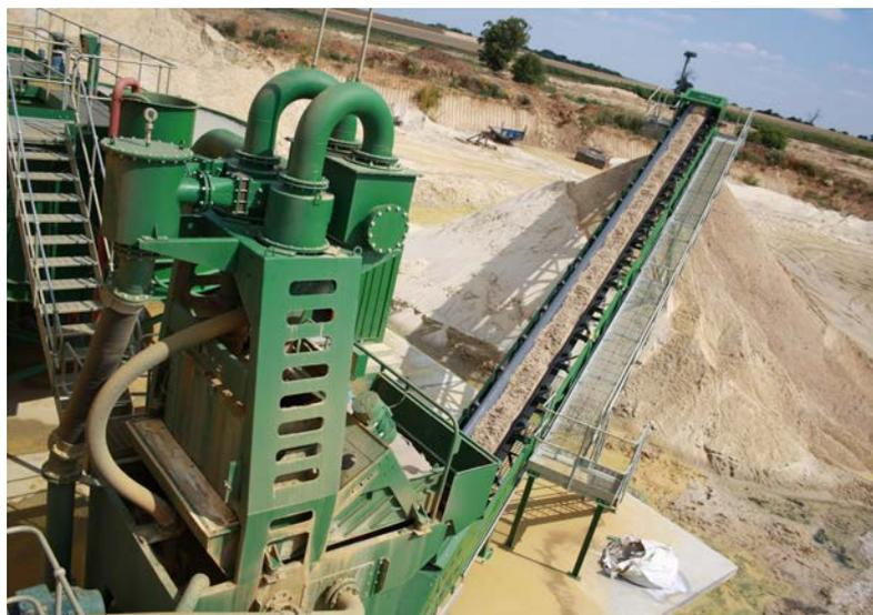
HydroCyclone technology facilitates highly accurate separation of silts and clays from the final washed sand product.
