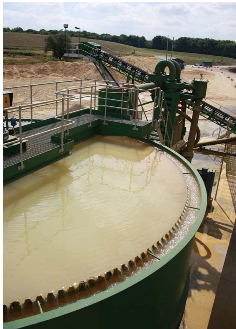
Clean water overflows the thickener and recycles to the AquaStore W372 water tank.
