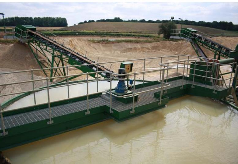
Excess fines are passed to the AquaCycle A400 water treatment system which allows high rate settlement of the fine particles to the bottom of the thickener tank.
