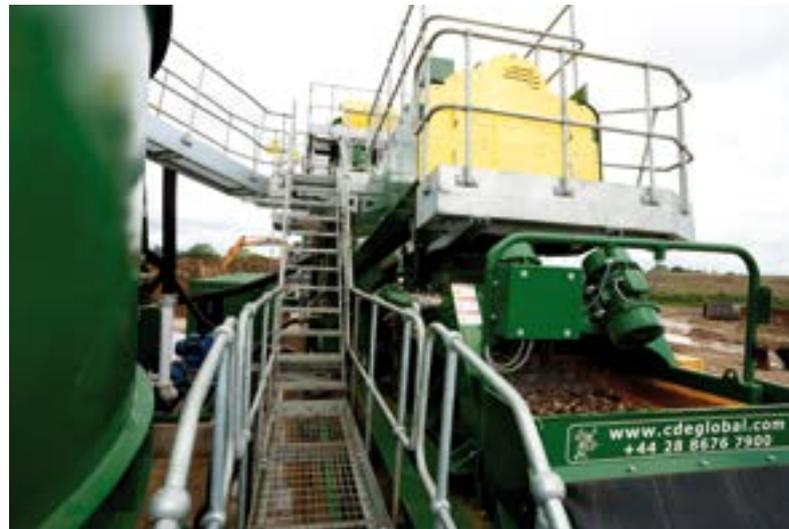
“As the scrubbed aggregates are discharged from the Rotomax they are delivered to a dewatering screen where they are given a final rinse before being sent to the aggregate sizing phase.”
