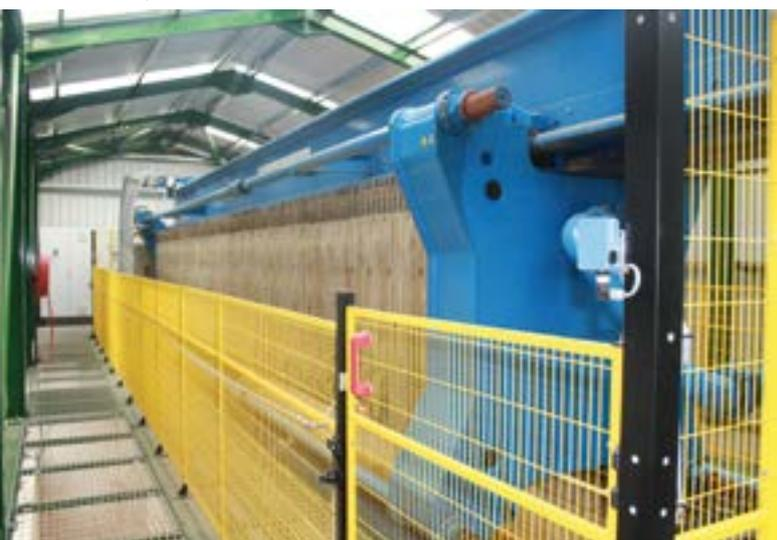
“ In this instance the filter press is made up of 140 plates which press the sludge at extremely high pressure to remove the maximum volume of water. The waste material is then compressed to a filter cake containing 90% dry solids content which is dropped from the filter press into a bay below. ”
