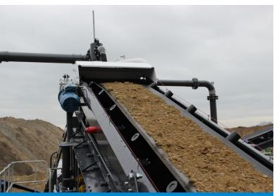
The sand and gravel feed is delivered to the M2500 washing plant by loading shovel and operates at 100 tons per hour. The plant accepts 0-100mm material with a grid on the feed hopper rejecting any oversize. The feed material is then delivered to the M2500 aggregate screening phase which is achieved using the integrated Prograde P2-75 rinsing screen.
