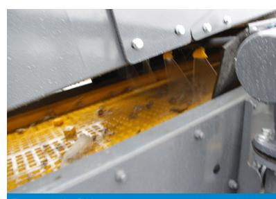
The top deck of this screen separates at +32mm and this material is sent to stockpile via one of the integrated wing conveyors. The bottom deck separates at 4-32mm and this material is then sent to the AggMax for scrubbing via the integrated Rotomax RX80 logwasher.
