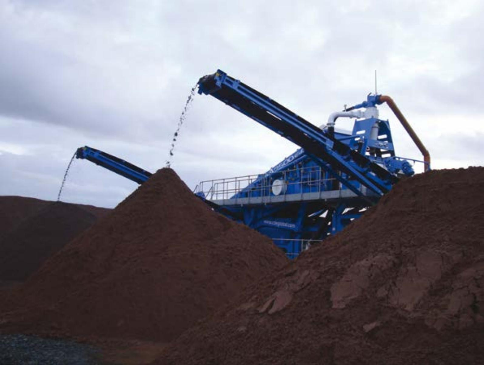
“ Once the material has passed through the Rotomax the scrubbed aggregates are discharged onto the integrated dewatering screen where they are sized into the final product gradings. These are subsequently stockpiled by three 15m mobile conveyors. ”
