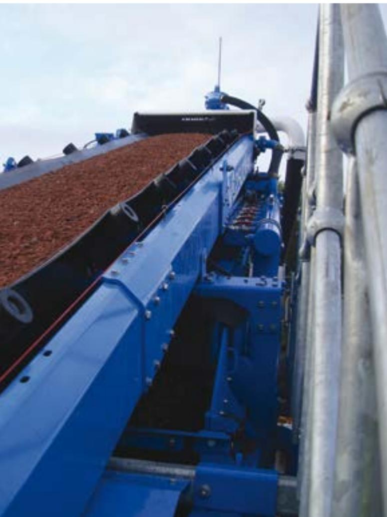
“ The feed material is delivered to the M2500 initially where initial screening separates the 0-6mm sand and grit fraction from the 6-40mm aggregate material. ”
