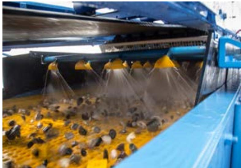
‘From the feed conveyor, material is discharged to the Prograde P2-75 double deck rinsing screen.’
