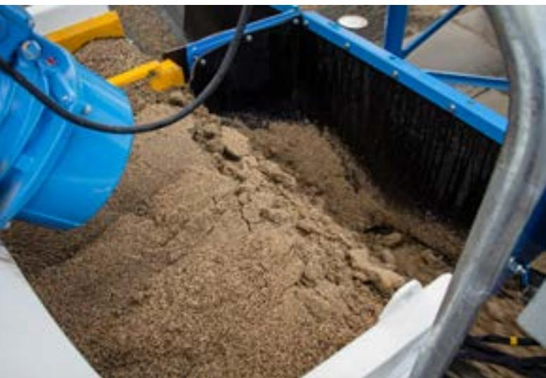
'The fine sand fraction is discharged via the cyclone underflow to the rubber lined feedbox which distributes the material evenly onto the second side of the dewatering screen. This maximises the screening area and ensures high efficiency dewatering.'
