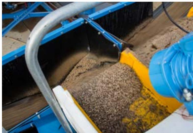
‘The 3-5mm material is transferred via jet pump to one half of the dewatering screen on the integrated EvoWash sand washing plant.’
