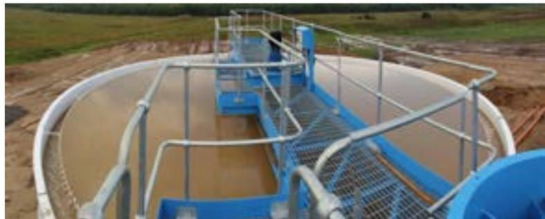
'The AquaCycle design allows for high rate settlement of these fine particles to the bottom of the thickener tank.'
