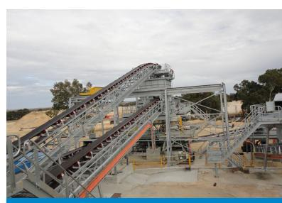
"We are now recovering and producing 25-30tph of quality sand with the total feed rate to the plant being 225tph. This technology has allowed us to increase efficiency by reducing the costs incurred through pond dredging to recover sand we had lost using the previous system".
