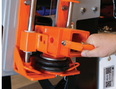
External servicing reduces confined space entry and eliminates reach-in maintenance, while facilitating faster blade replacement.
