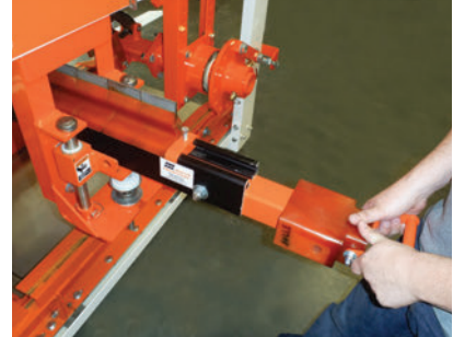
The slide-out design is engineered so the blade cartridge can be accessed safely and replaced by a single worker.
