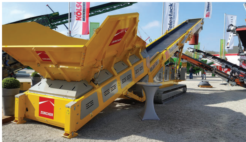
LF514 displayed at Bauma 2016 which was sold to Zurcher in Germany – a large German rail infrastructure company who used the LF to load rail cars with railway ballast.
