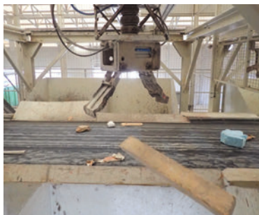
The picked wood is dropped into a specific chute and sorted
