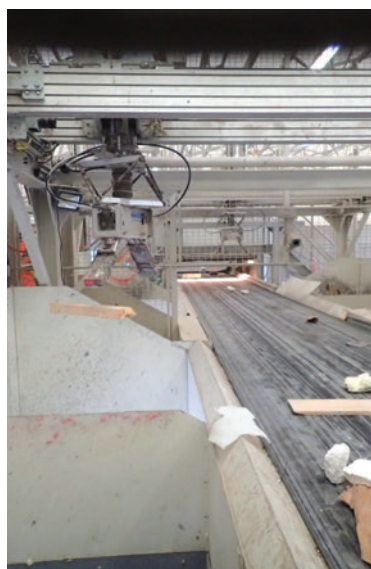
The picked wood is dropped into a specific chute and sorted
