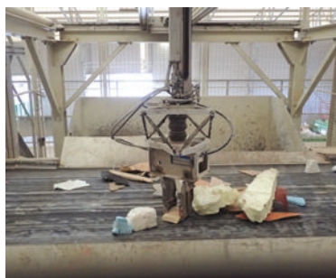
The robot identifies a piece of wood and grasps it
