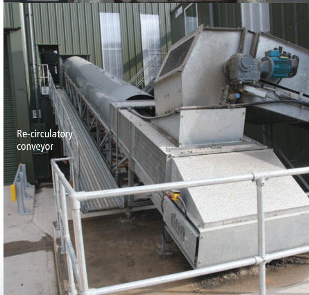
Re-circulatory conveyor, feed end onto primary conveyor
