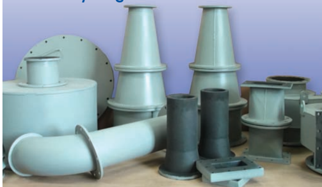
Rubber lined components for a sand washing plant.
