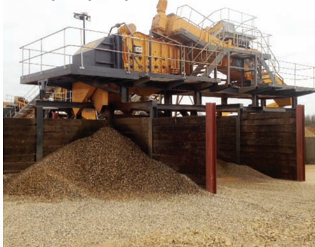
BWR300 Washing System (scrubbing , rinsing & sizing )
