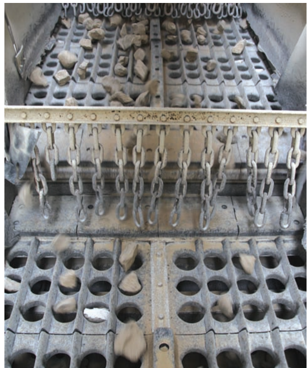
Hewitt Robins V-16 2.5 x 6.0 double-deck heavy duty selector screen
