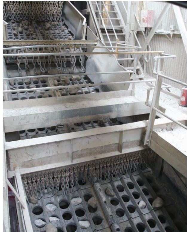
Hewitt Robins V-16 2.5 x 6.0 double-deck heavy duty selector screen
