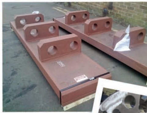
Fabricated wall liner for a metal recycling shredder, the impact wall is 120mm thick in Hardox 400/450.
