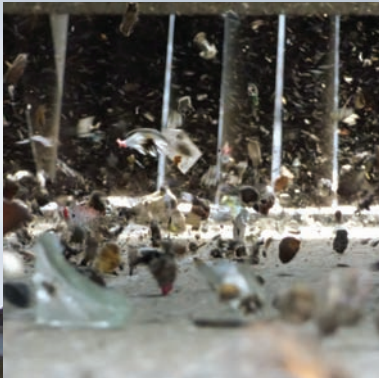
The air separation process in the Westeria AirBasic
