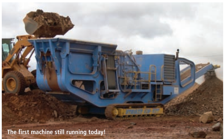
Primary JM1310 jaw crusher installed into a quarry in Western Australia
