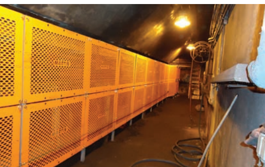
Martin Conveyor Guards simplify conveyor guarding, allowing easy inspection, while protecting workers from moving components and pinch points.
