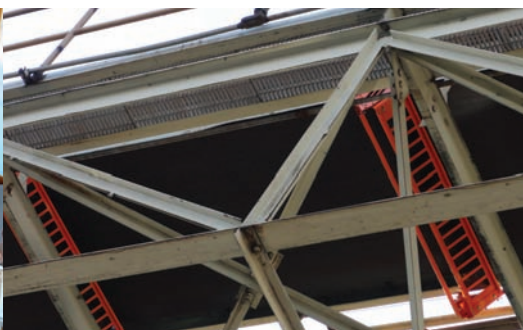
The Return Roller Basket was developed to prevent a return roller from falling in the event of a mechanical failure.
