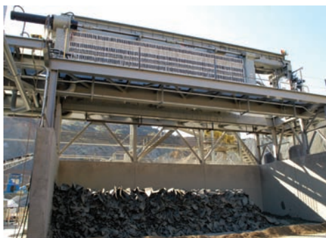
McLanahan Filter Presses eliminate the need for settling ponds while providing reusable wash water and freeing up valuable resources.
