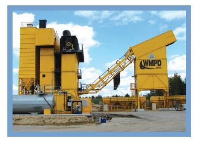
extensive range of hot storage systems. These include a compact four silo cluster, which allows the discharge from all four silos to a single truck loading point; this offers the opportunity to use one weighbridge for vehicle loading.
