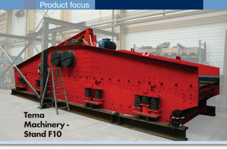
Tema Machinery will be exhibiting a wide selection of equipment which will include a 2.7m wide x 10m long double deck linear motion screening unit which will take centre stage on the stand. This machine is one of 12 similar size units to be installed at Lafarge Mountsorrel, and it will be fitted with Tema Isenmann Polyurethane screen panels.
