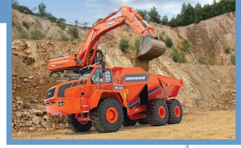
Powered by the 6-cylinder Scania DC13 Stage IIIB compliant diesel engine with a gross power output of 368 kW (500 HP) at 2100 rpm, the new DA40 offers a 10% increase in engine power compared to the previous MT41 model.
