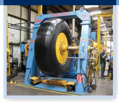
process of retreading earthmover and mining tyres will always generate waste', what Kal Tire have indentified and reacted upon is that this discarded material (primarily rubber compound 'crumb' buffed from the tyres prior to retreading or repair) may have a secondary use.
