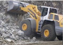
RUD's innovative tyre protection chains ensure that customers in demanding working environments can operate effectively and safely. Working machines in areas with fire and hot slag conditions can be very dangerous and lead to loss of equipment through burnt tyres. With RUD's tyre protection chains they offer specially developed hardened forged wear links which guarantee optimal tyre protection in the use on hot and burning surfaces.
