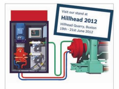
▲ A typical drive consists of a Hägglunds motor which will provide the torque required. A power unit with a variable displacement pump/motor set and necessary tank, filters and instrumentation is also included in addition to a control and monitoring unit and the inter-piping. The arrangement is versatile and flexible which enables customisation to suit the exact requirements of the application and environment.
