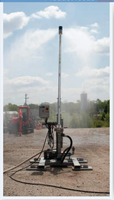
Just 10 PSI of water pressure is required from the supply hose when using the integrated booster pump, giving the DB-M an output as high as 24 GPM at 200 PSI. An in-line 30 mesh filter stops any solids 600 microns and larger, and the manufacturer recommends that it be used at all times. If using potable water, nozzles can be inspected just once a year.
