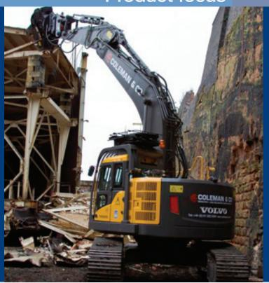
The EC305C rewrites the rules on short radius excavator design. As the third and largest model in the ECR range, it offers best in-class lifting capacity, stability, digging force and fine control. On 800mm tracks, the upper structure swings outside its own track width by just 80mm.
