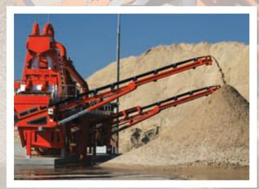
Once material has been delivered to the M2500 E4X the feed conveyor delivers the material to a double deck ProGrade P275 rinsing screen fitted with wire mesh on both decks. The +22m material is removed by the top deck and the 15-22mm by the bottom deck and these products are stockpiled by the integrated 9m wing conveyors.
