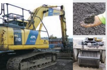
A Rotar 900R screener bucket has helped a Nottingham-based company overcome a 17-year old materials processing problem, converting a tricky and sticky waste into a saleable commodity.
