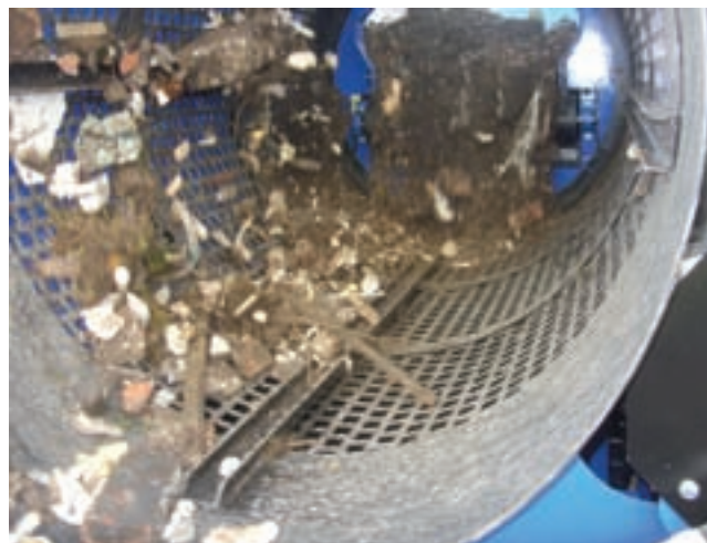
Ultra T-1500 taking cleaning fines from skip waste at 30mm
