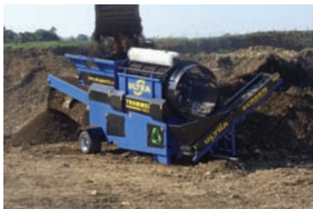
Ultra T-1500 cleaning contaminated topsoil at 60 tph
